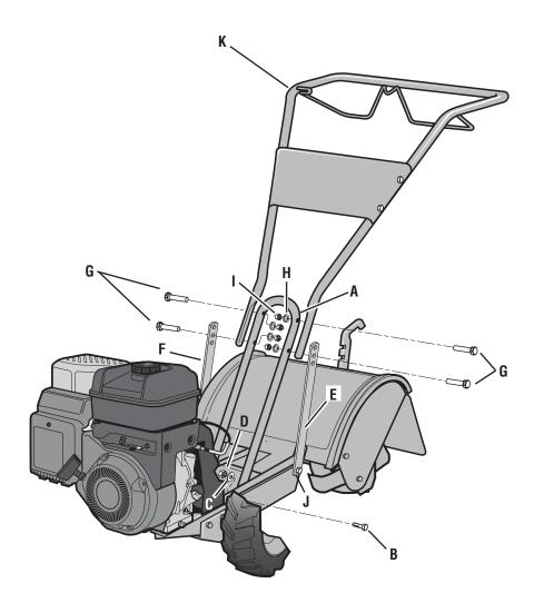
Fig. 2-2: Attach handlebar.
